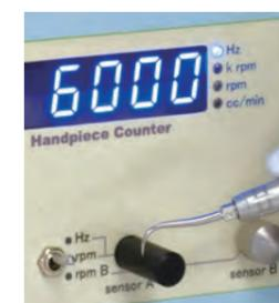
As the measurement object and the sensor do not have to touch, Q-unit determines the handpiece performance safely and simply.
