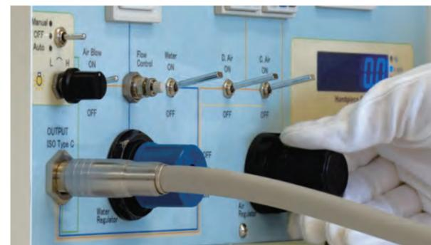
Q-unit is equipped with useful functions for different test, inspection, and maintenance works: on-off controls for driving air, cooling water, chip air, and illumination. In addition, Q-unit has an air-blow system to discharge cooling water remaining inside of the handpiece after use.
