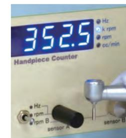
Q-unit has two sensors to measure number of revolution and frequency.
